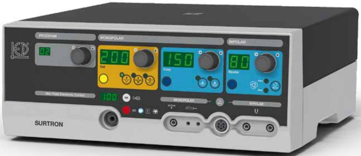
SURTRON® 200 is a high frequency electrocautery equipment which is suitable for light and medium surgery.
